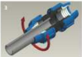
Fully coil back the nut.
