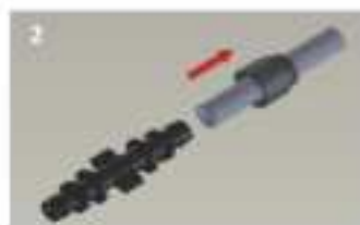
Pull the coupling nut up to the end of the pipe
